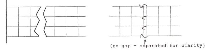
The next step is to form the curved shape of the basket by progressively shortening the lengthwise wires with a crimping tool. Doug used a tool made by adapting an old leather-punch pliers but ordinary pliers could probably be adapted successfully.
